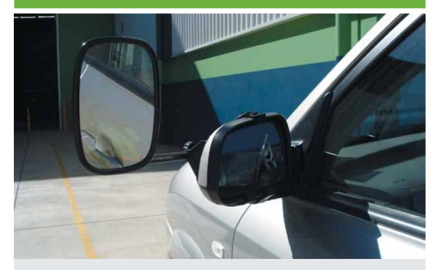
Reich made quite a name for themselves when they developed the Move Control Series of caravan movers. Now these innovative Germans have produced a range of towing mirrors designed to give you a vibration free, hassle free & obstruction free towing experience. They feature a turn knob which controls the length of the straps, ensuring maximum tightening security onto the existing car mirror.
